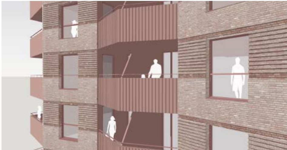
Metal balcony design and brick corbelling
